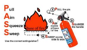
**SWEEP** the nozzle from side to side at the **base of fire** until it appears to be out then **watch** the fire area for possible re-ignition.
