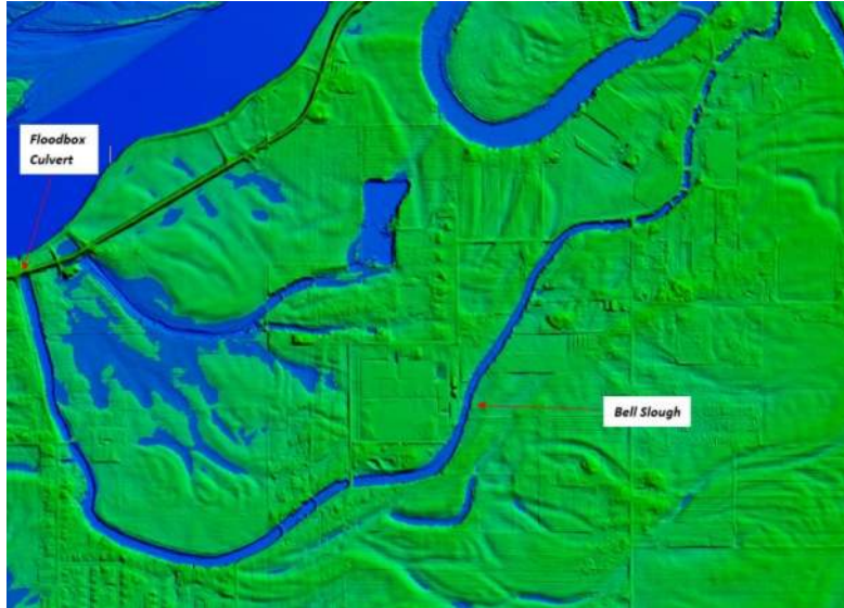
Figure 5-9: Water Level in the Bell Slough and Surrounding area at 10.15 m Elevation
