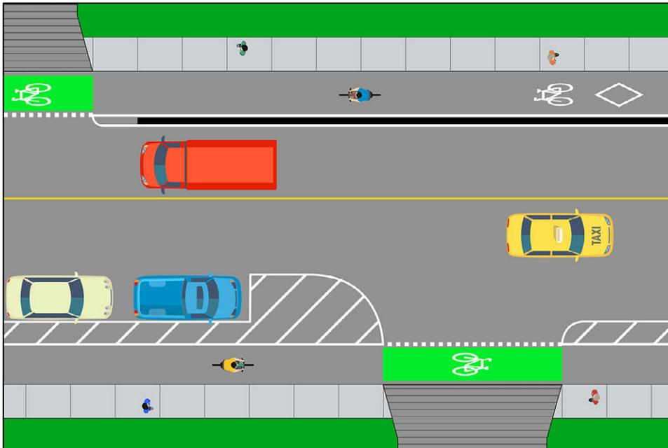
**Figure 5.3 – Bicycle lane with localized protection (Vancouver)**
